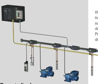
With the appropriate **podis** \* /**gesis** \* installation systems Wieland power bus concepts are suitable for setting up distributed solutions for drive control on technical conveyor systems. Possible applications range from pure power-distribution via fieldbus interface to motor
