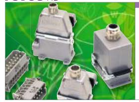
**revos** HD is designed specifically for multi-pole pluggable connectors. The robust housings provide space for contact inserts with 15 to 64 poles and are designed for currents up to 10 A (in compliance with DIN EN 17 5301-801). **revos** HD proves its strengths in mechanical and systems engineering, in escalators, small motors and injection molding machines.
