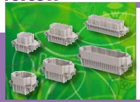
High contact density in a very limited space – this is what **revos** DD space-saving contact inserts offer. The inserts are compatible with BASIC housing sizes 6/6H-, 10/10H-, 16/16H-, and 24/24H. They are connected with reliable, twisted 1.6 mm crimp contacts and a connecting range of 0.14 - 2.5 mm<sup>2</sup> at a rated voltage of 250 V.
