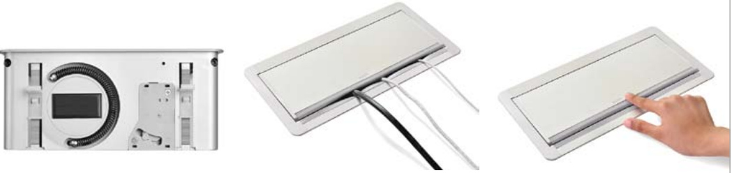
Mounting with the click-stop mechanism reduces installation to no time. The NETBOX Axial Comfort can be utilised in a 'closed' position thanks to the rubber lips which allow cables to run through. The unit's unique spring mechanism allows for easy access at the push of a finger.
